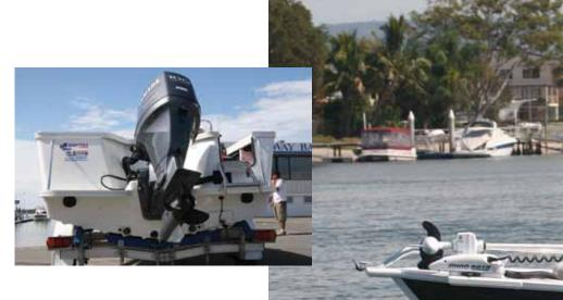
**Power:** The 530 Top Ender is rated for a single outboard up to 115hp. That's a pretty good call because our test boat got along pretty well with a 100hp Yamaha motor. The following were the GPS speeds attest:
